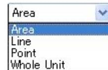
Position: Scanning position(s) will be specified here. The scanning positions will be specified in different ways according to the scanning mode.
