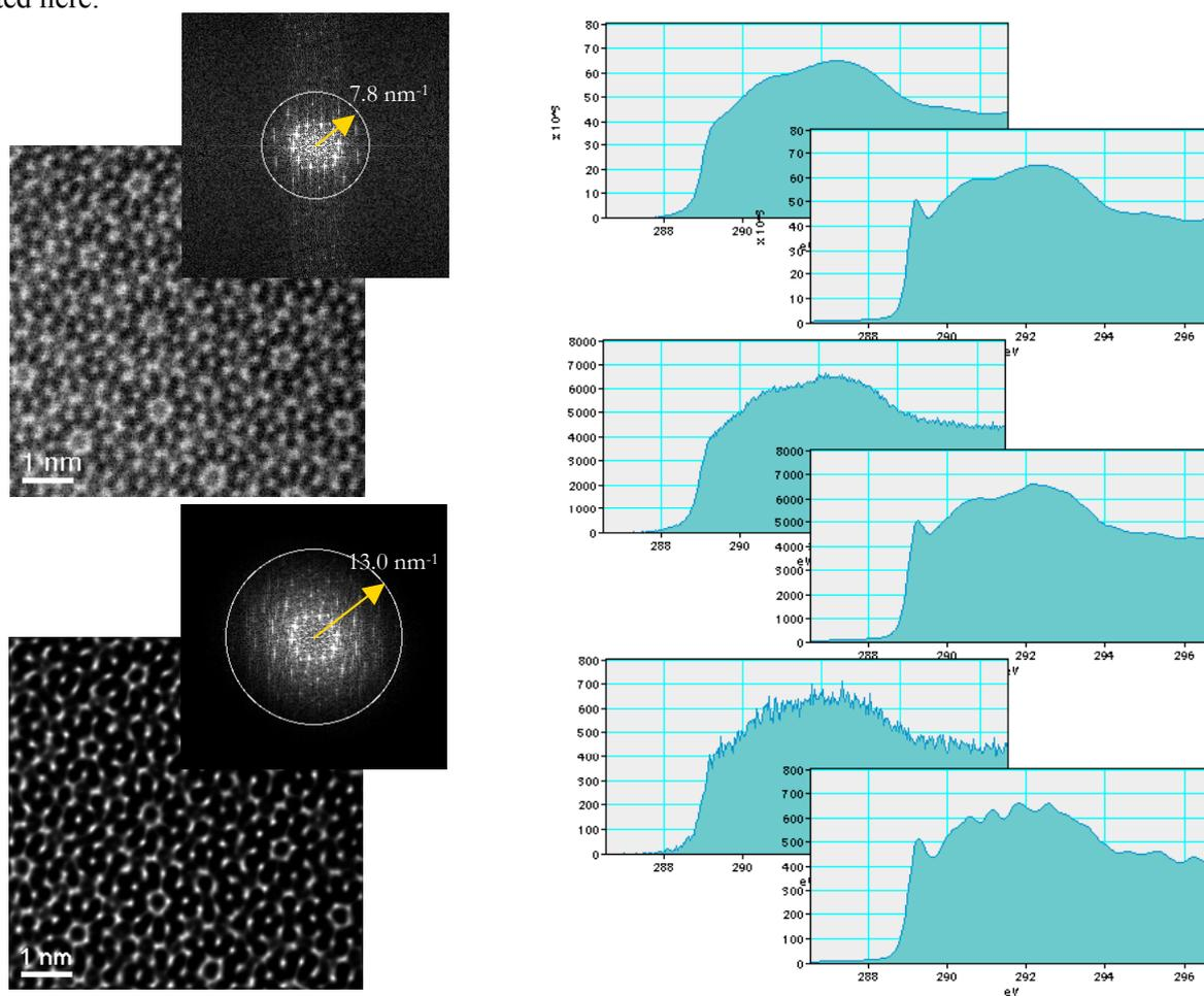
**(Left) Fig. 1.** Original quasi-crystal image (top) and deconvoluted MEM image (bottom) with a calculated probe assuming  $z = -45$  nm (at 64 cycles). Here, the resolution of the original image is about  $7.8 \text{ nm}^{-1}$ , while the resolution of the deconvoluted image is about  $13.0 \text{ nm}^{-1}$ . The original image was obtained by E. Abe using JEOL 2010F (200 kV, Cs: 0.5 mm, probe forming angle:  $\sim 12$  mrad, ADF detector:  $50 - \sim 110$  mrad).
