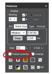
By choosing this option, HoloLive! no longer hunts for the sideband in the live FFT, it just continues to use the same carrier frequency  $\mathbf{q}$ . There is a slight increase in speed. Unticking the option just lets HoloLive! go back to automatically detecting the sideband.
