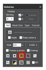
**Technical note:** the default for HoloLive! is a reference area at the centre of the image, rotated parallel to the hologram fringes. This can be modified in the **HoloLive...Reference Area...Settings.** These settings can be accessed via the HoloLive! menu or by pressing CTRL while clicking on the **Reference Area** button.
