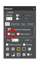
The phase variation across the field of view is much smaller. Click and unclick **Apply** to see the improvement. Ideally, there should be no phase variation on correction (apart from the noise from the counting statistics). As is often the case, the reference image was acquired a bit later in the day when the imaging conditions had changed slightly.
