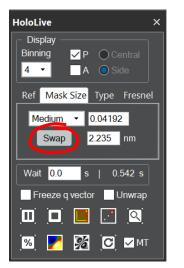
**Technical note:** the choice of sideband is important for subsequent quantification. Our convention is that the sideband pointing towards the reference wave (usually the vacuum) should be chosen. In that case, the phase is positively proportional to the mean-inner potential of the material. A positive phase gradient means increasing sample thickness. Have a go but remember the delay.
