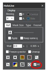
**Technical note:** In fact, MT stands for "Multi-Threading". By programming in parallel certain operations in the sequence (FFT, masks, reference) the delay between successive phase images is reduced. However, the time to create the first phase image in a sequence is always the same and corresponds to the delay time without **Turbo Boost**.
