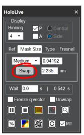
**Technical note:** the choice of sideband is important for subsequent quantification. Our convention is that the sideband pointing towards the reference wave (usually the vacuum) should be chosen. In that case, the phase is positively proportional to the mean-inner potential of the material. A positive phase gradient means increasing sample thickness.
