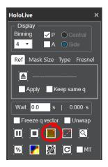
Technical note: the default for HoloLive! is a reference area at the centre of the image, rotated parallel to the hologram fringes. This can be modified in the HoloLive...Reference Area...Settings. These settings can be accessed via the HoloLive! menu or by pressing CTRL while clicking on the Reference Area button.
