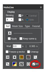
**Technical note:** In fact, MT stands for "Multi-Threading". By programming in parallel certain operations in the sequence (FFT, masks, reference) the delay between successive phase images is reduced. However, the time to create the first phase image in a sequence is always the same and corresponds to the delay time without **Turbo Boost**.
