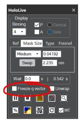
By choosing this option, HoloLive! no longer hunts for the sideband in the live FFT, it just continues to use the same carrier frequency **q**. There is a slight increase in speed. Unticking the option just lets HoloLive! go back to automatically detecting the sideband.
