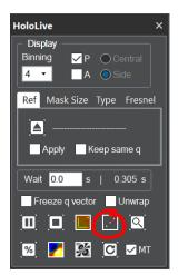
**Technical note:** it is too time consuming for HoloLive! to calculate a live Power Spectrum (which includes masking in real-space). The **FFT** button shows the modulus of the FFT of the hologram (which had to be calculated anyway for the phase image). You will therefore notice streaking of the spots. Purists can see the *static* Power Spectrum using **HoloLive...Power Spectrum**.
