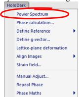
**Technical note:** in HoloDark, the image does not have to be a power of two in size (e.g. 512 by 512). However, streaks may appear in the power spectrum if greatly different in size from a power of two.
