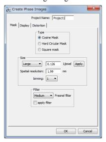
**Technical note:** in general we recommend the *Cosine Mask*. The *Hard Circular Mask* and *Square Mask* have been included as an option. The most important parameter is the mask size which determines the spatial resolution of
