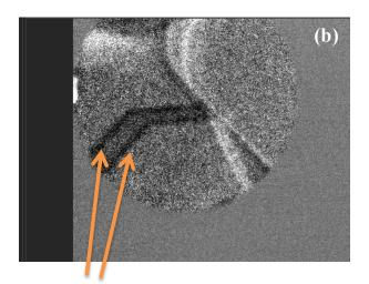
Two shadows of the crystal due to the sample movement caused by the beam tilt
