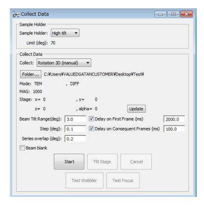
**Fig. 12** Data collection dialog box that appears after choosing "**Collect Data....**" in the pull-down menu of EDT/Collect in Fig. 2.
