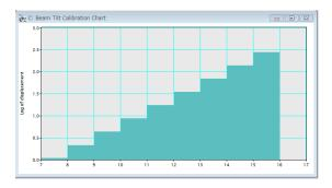
**Fig. 8** A relation between a parameter for coil current, CV-value, and tilted electron beam position in log vs. log axis.
