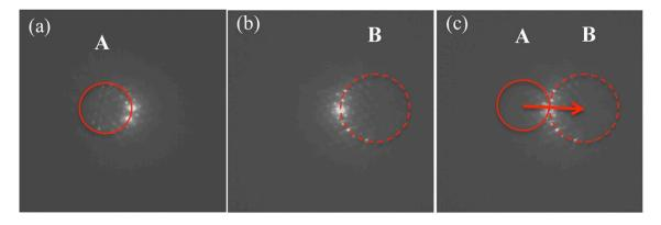
**Fig. 17** a: Sample holder is slightly tilted towards the (-) direction from an exact zone axis. Laue circle "A" can be seen. **b**: Sample holder is tilted towards the (+) direction slightly. Laue circle "B" is seen. **c**: indicates Laue circles "A" and "B" on a same picture.
