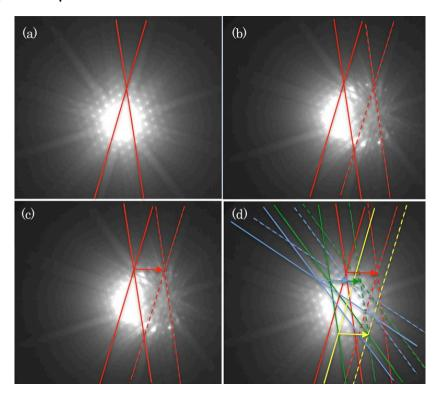
**Fig. 16 a, b, c, d,** diffraction-pattern from a crystal specimen at relatively thick position. **a** and **d** show the Kikuchi-pattern before the sample holder tilt, **b** and **c** show the pattern after the holder tilt.
