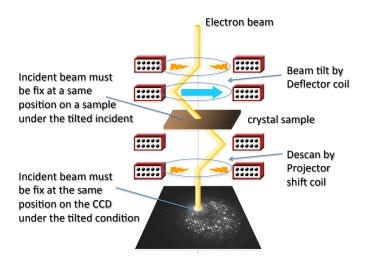
Fig. 1 Ray path diagram of EDT/Collect experiment
