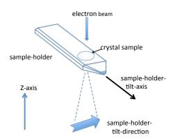
Fig. 18 Relation between sample-holder-tilt-axis and sample-holder-tilt-direction
