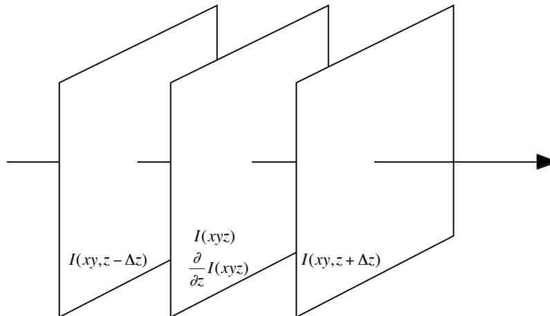
**Figure 1.** Three images taken with the same defocus step. The phase distribution at the middle plane is determined from image intensities at three image planes by using the Transport of Intensity Equation.
