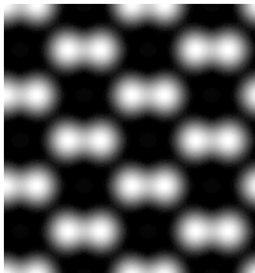
Simulated HAADF image for GaAs [011]
